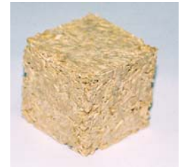
Fig. 4 – Concrete with hemp hurds, metakaolin, lime and waste paper pulp.
