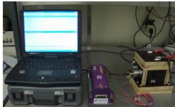
Figure 1. Setup for Ultrasound pulse velocity and electrical resistivity measurements: a) pc; b) DataTaker; c) electrical cable connection for temperature measurement; d) polywoud cubic box; e) transducers; f) electrodes
