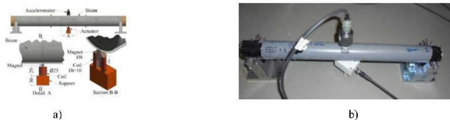
Figure 2. a) Schematic view of custom made non-contact electromagnetic actuator attached to an EMM-ARM beam [units: mm] [14]; b) EMM-ARM beam.
