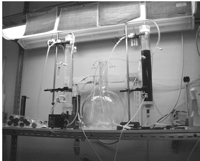
Figure 5 – The former separation columns adapted to act as bioreactors.
