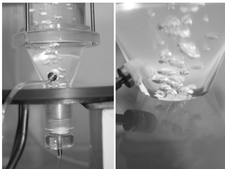
Figure 10 – Left image: the lower cone with primary inlet/outlet; right image: detail of gas injection.
