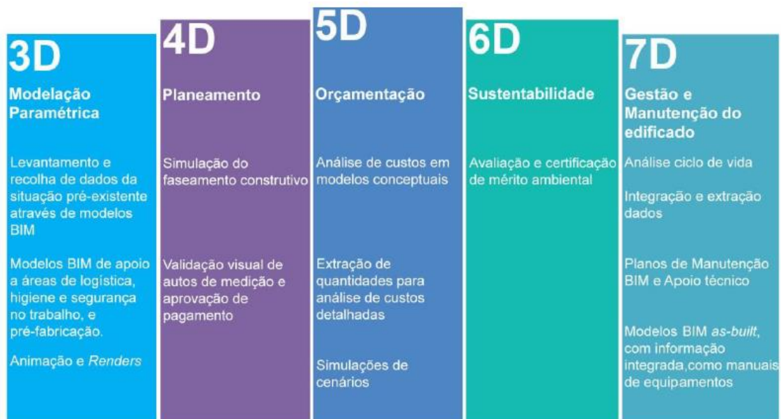
Figura 7 – BIM 3D a BIM 7D (Adaptado: (Hughes, 2013))
