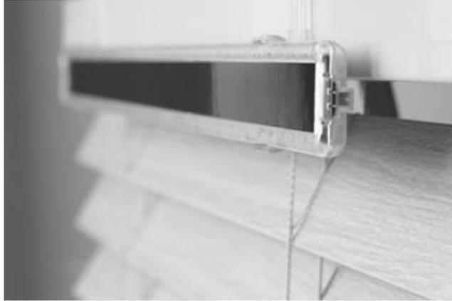
**Figura II-2:** Painel solar da *MySmartWindow*.
