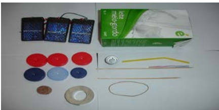
Figure 1. Materials used by a group of students to build a solar car
