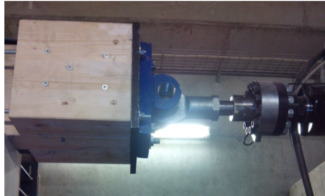
Figure 6. Detail of the fixation of the load-cell to the top beam responsible for the application of the loading protocol.
