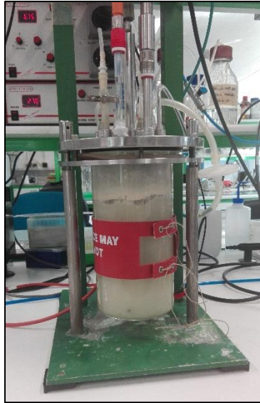
Figure 3.1 Stirred tank bioreactor (BIOLAB, B. Braun, Germany) with optimized medium for lipase production.
