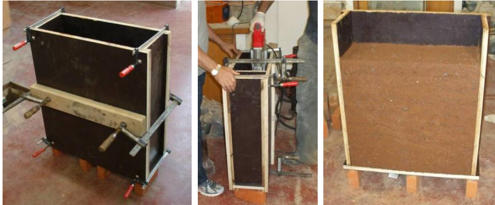
Figure 4: Manufacturing of the URE wallets.
