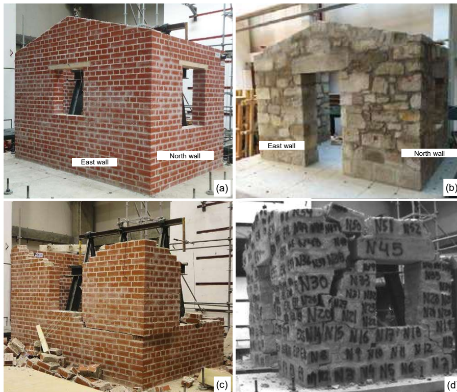
124 Figure 1. Brick House (a,c) and Stone House (b,d) specimens before the beginning of the shake table tests (a,b) and at collapse (c,d) 125 (Candeias et al., 2016).
