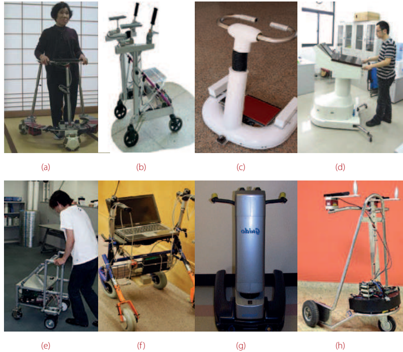
Figure 1. Smart walkers. (a) JARoW [6]; (b) Simbiosis [5]; (c) i-go [7]; (d) Ye et al. [8]; (e) RT walker [9]; (f) i-walker [10]; (g) GUIDO [11]the Assistive Mobility Device (AMD); (h) UFES [12].
