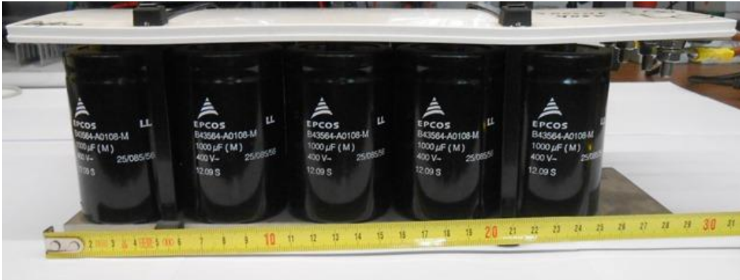
Figure 5.20 – DC-bus implemented, composed by a pack of capacitors resulting in a total capacity of 10 mF and a maximum voltage of 450 V.
