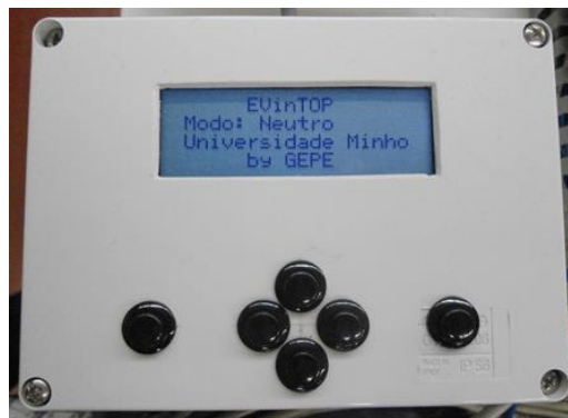
Figure 5.16 – Human-Machine Interface (HMI), developed in the GEPE, used to provide an easier interface with the control system.
