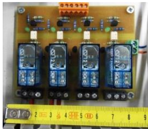
Figure 5.12 – PCB developed in the GEPE for control the actuation of the pre-charge circuit.
