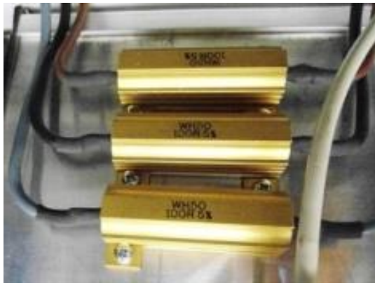
Figure 5.24 – Resistances used for the pre-charge circuit (each one with a resistance value of 100\ \Omega \pm 5\% , 50 W).
