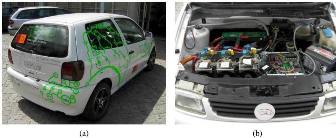
Figure 1.13 – Carro Elétrico Plug-In da Universidade do Minho (CEPIUM), the EV developed in the University of Minho: (a) Overview; (b) Power electronics converters and control system implemented under the hood.
