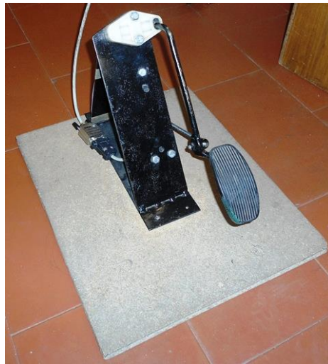
Figure 5.15 – Electronic accelerator pedal used for setting the torque reference in the motor drive mode.
