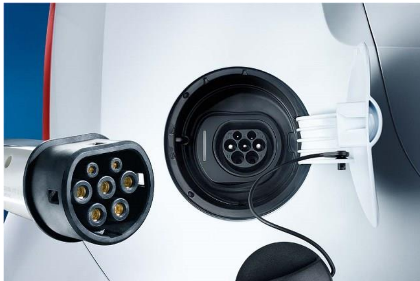
Figure 1.9 – Charging socket and connector used in the Volkswagen e-Up! (gently provided by Volkswagen Portugal – Siva ).
