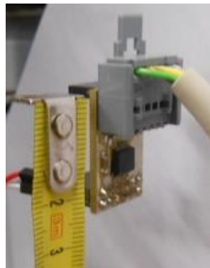
Figure 5.14 – PCB developed in the GEPE for interface between the position sensor with the DSC.
