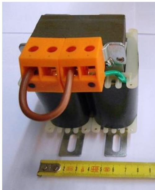
Figure 5.23 – Inductor used to implement the extra input filter of proof-of-concept prototype.
