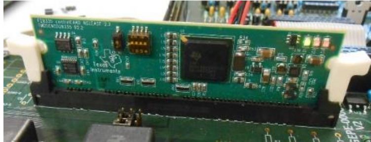
Figure 5.9 – ControlCARD provided by Texas Instruments to interface with the DSC TMS320F28335 .
