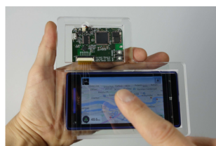
FIGURE 2.23: Gesture recognition on mobile device [35]
