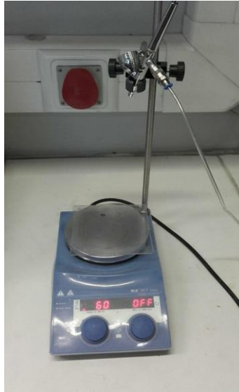
Figure 17: Equipment used to produce PVA composite films
