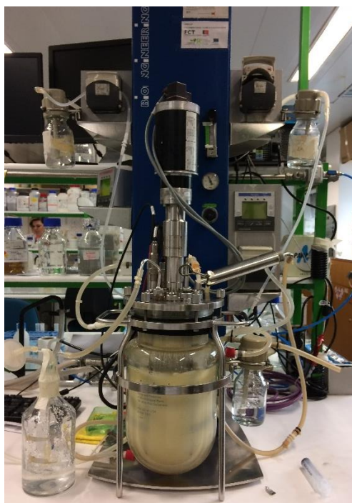
Figure 3 – Bioreactor (RALF PLUS SOLO, Bioengineering, Switzerland) with production medium.
