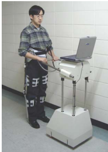
Figure 22: Tendon-driven exoskeletal power assistive device and caster walker (Kyoungchul Kong and Doyoung Jeon, 2005).
