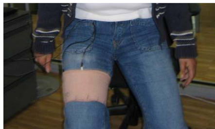
(a) The force sensor and the elastic band used in the experiments. (b) One of the subjects with the band on the leg doing squats.
