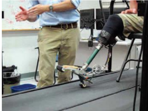
Figure 10: Tethered prosthesis testbed developed at Carnegie Mellon University, Pittsburgh, USA (Cherelle et al., 2014).
