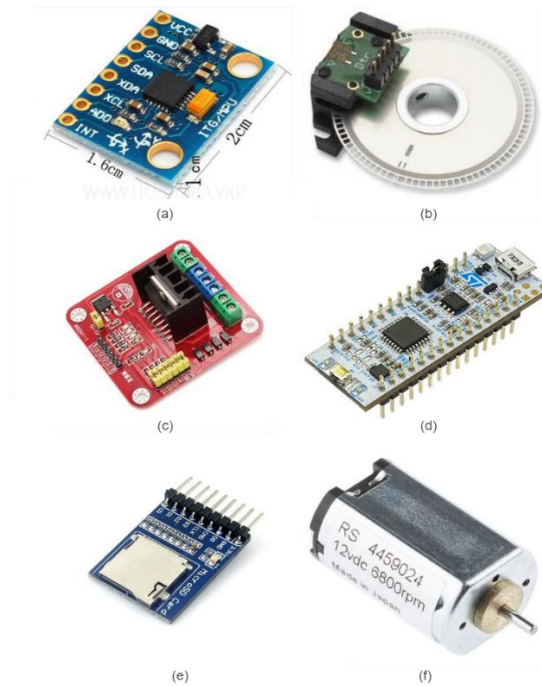
Figure 53: Required Hardware: (a) MPU 6050; (b) Incremental Encoder; (c) Motor Driver L298N; (d) STM32F303K8 Nucleo; (e) SD Card Reader; (f) Motor
