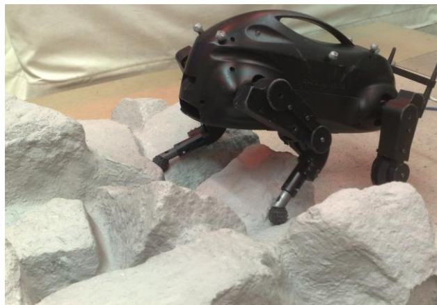
Figure 6: The quadruped robot LittleDog and a sample terrain to be crossed (Buchli et al. , 2009)
