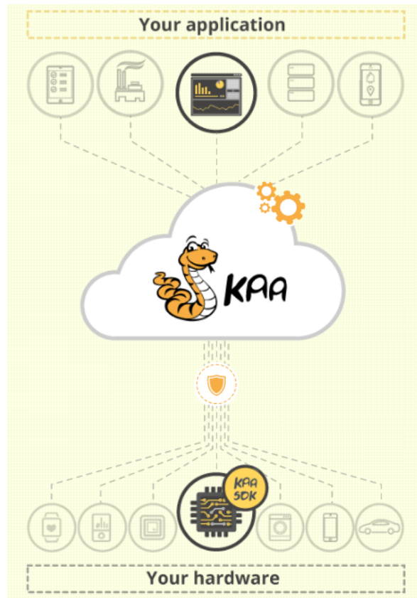
Figure 8: Overview of the Kaa platform as a middleware between the hardware devices and the application layer. The devices are provided with Kaa SDKs to securely communicate with the server, which integrates several applications, such as data management and analytic systems [22].
