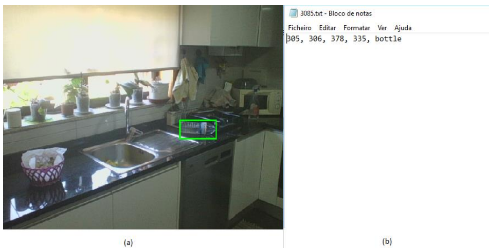
Figure 30 - Acquisition of the dataset where (a) is the raw image with the bounding box and (b) is the corresponding ground truth information, namely, the box coordinates (xmin, ymin, xmax, ymax) and the respective class. Note that the coordinates presented in (b) is just an example, as it is not the corresponding box presented in (a)
