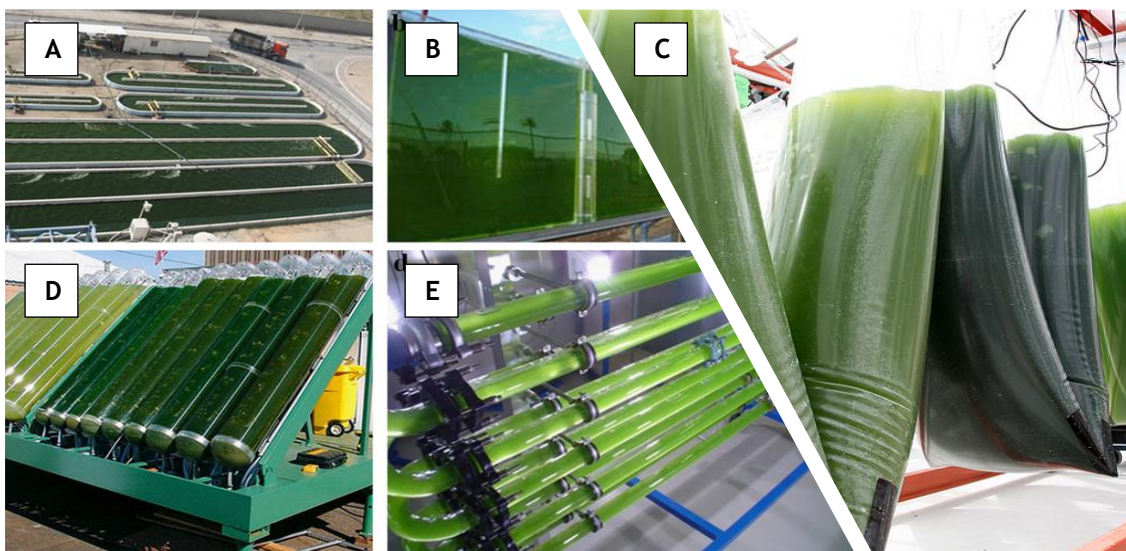
Fig. 2: Open and closed systems to microalgae culture. A - Open pond system; B - Flat panel system; C - Bag-type photobioreactor; D - Vertical tubular system; E - Horizontal tubular system.
