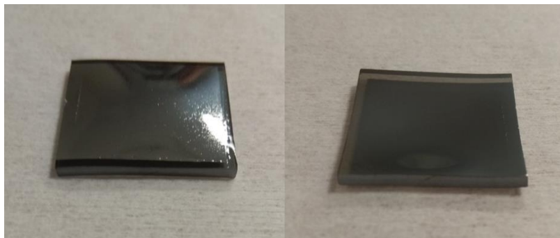
Figure 5.1 - Sample (glass/Mo) after heating at 570\text{ }^{\circ}\text{C} .
