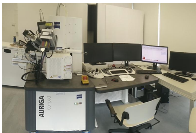
Figure 3. 7 - High-Resolution Field Emission Scanning Electron Microscope with Focused Ion Beam (FIB – SEM) [58] .
