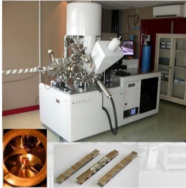
Figure 16: System of analysis of surfaces by electron spectroscopy: XPS (Kratos Axis Ultra HAS) [113].
