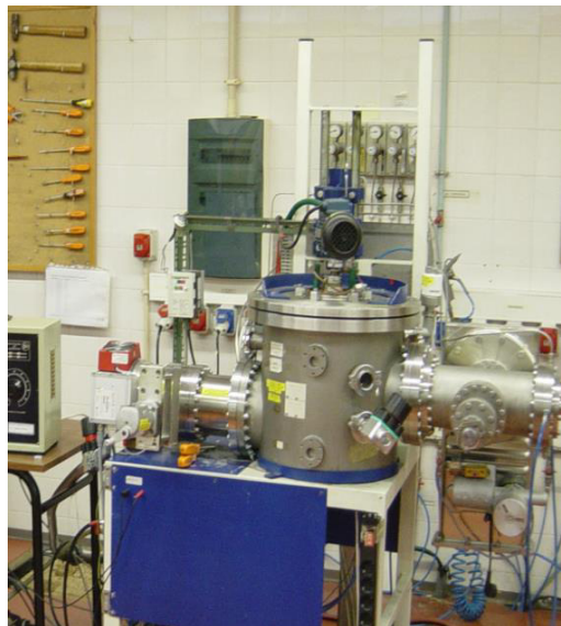
Figure 9: The used DC sputtering chamber for coatings deposition.
