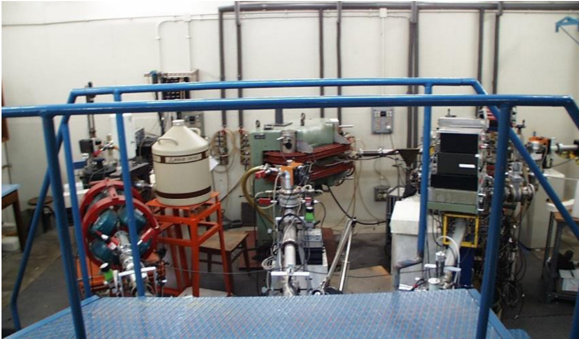
Figure 14: A 2,5 MV Van de Graaff accelerator with three experimental beam lines, with all the relevant ion beam techniques available: RBS, PIXE, NRA, Channelling, ERDA and NRB [110].
