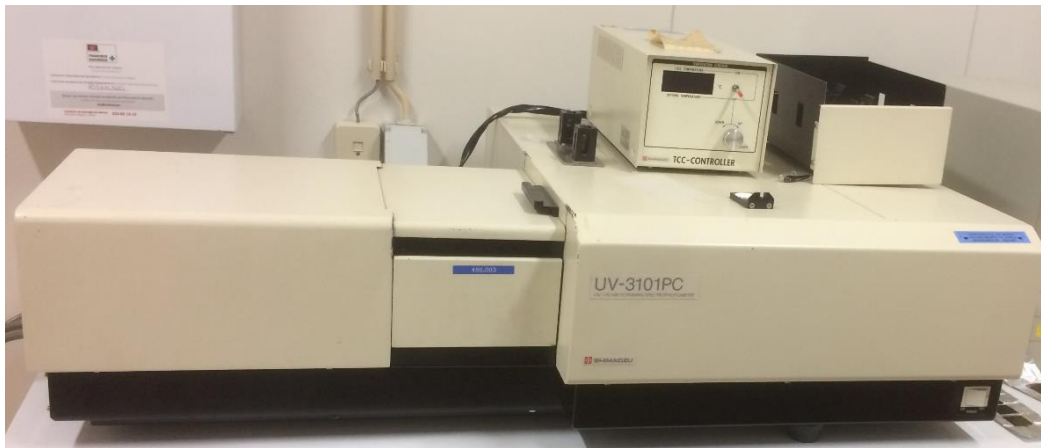
Figure 12: The Shimadzu PC3100 spectrophotometer used for transmittance (T) and the reflectance (R).
