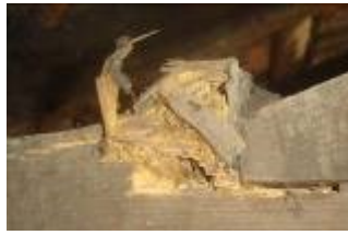
a) Damage at 2550 kg of loading
