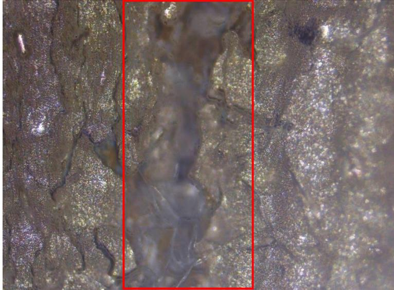
*Figure 5 Cracks formation on CO plasma 825 sample 5x magnified*
