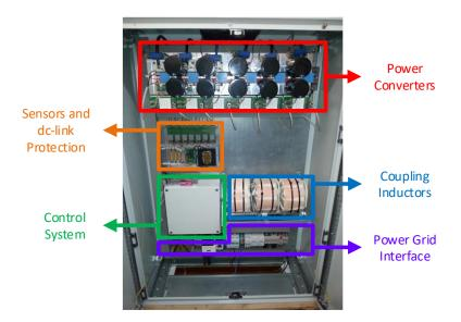
Fig. 4. Laboratory prototype of the developed VSD.
