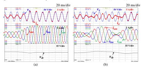
**Fig. 10.** Results obtained for the motor driving a 5 Nm load during: (a) Acceleration from 600 rpm to 800 rpm; (b) Deceleration from 800 rpm to 600 rpm.
