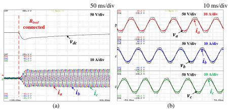
Fig. 6. Active rectifier operation with a 25  $\Omega$  load connected to the dc-link: (a) Transient state dc-link voltage and power grid currents; (b) Steady state power grid voltages and currents.
