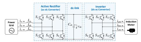
Fig. 1. Proposed system for the VSD.
