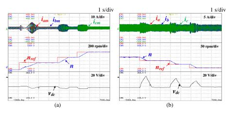
Fig. 9. Results obtained in the operation of the motor for a constant load of: (a) 3 Nm; (b) 5 Nm.
