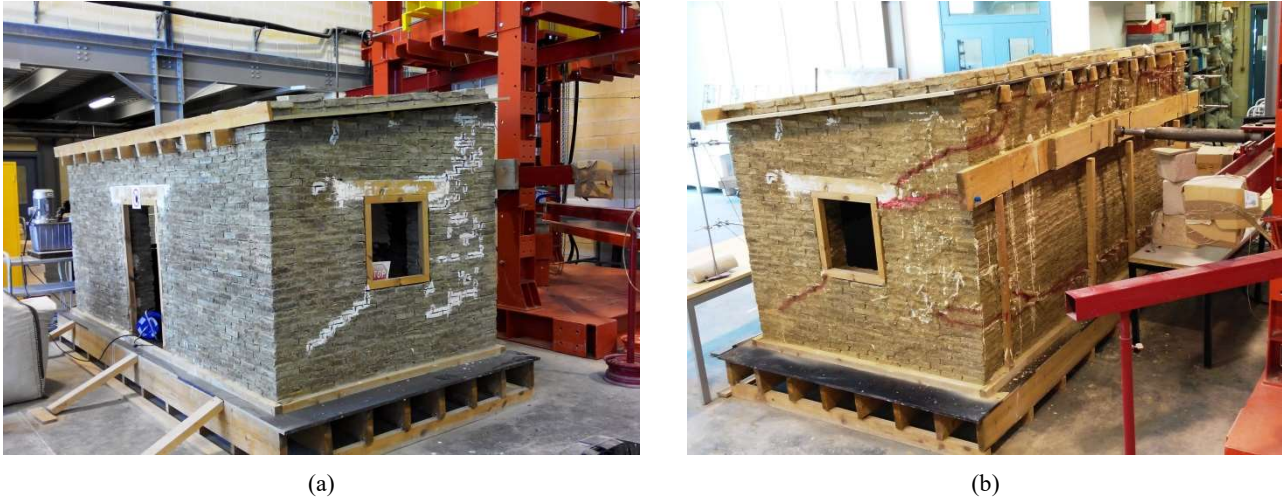
Figure 1. Front (a) and rear (b) views of the tested scaled adobe building. In the rear view of the structure, the load imposition timber beam and the hydraulic jack used for exerting horizontal forces are shown.
