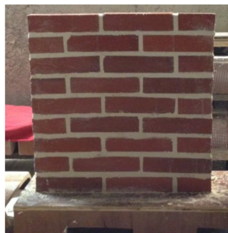
279 280 Fig. 2. Unreinforced masonry specimens (URM). Sizes in mm.
