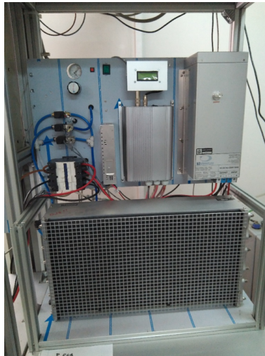
(a) Fuel cell (Horizon 5000W)
