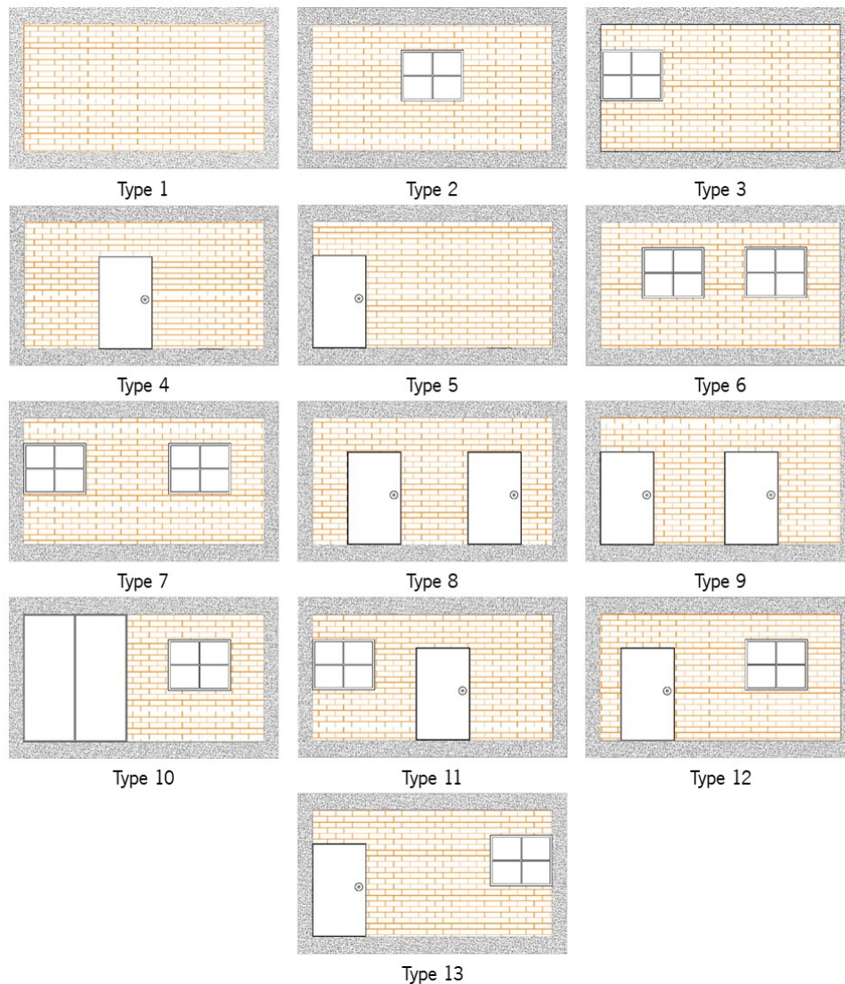
Figure 3: Masonry infill wall types
