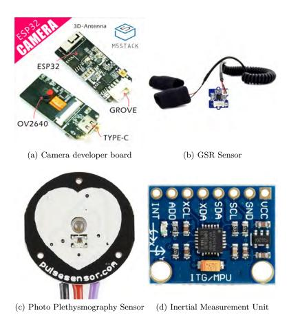
Fig. 1: Sensors used in the wristband.
