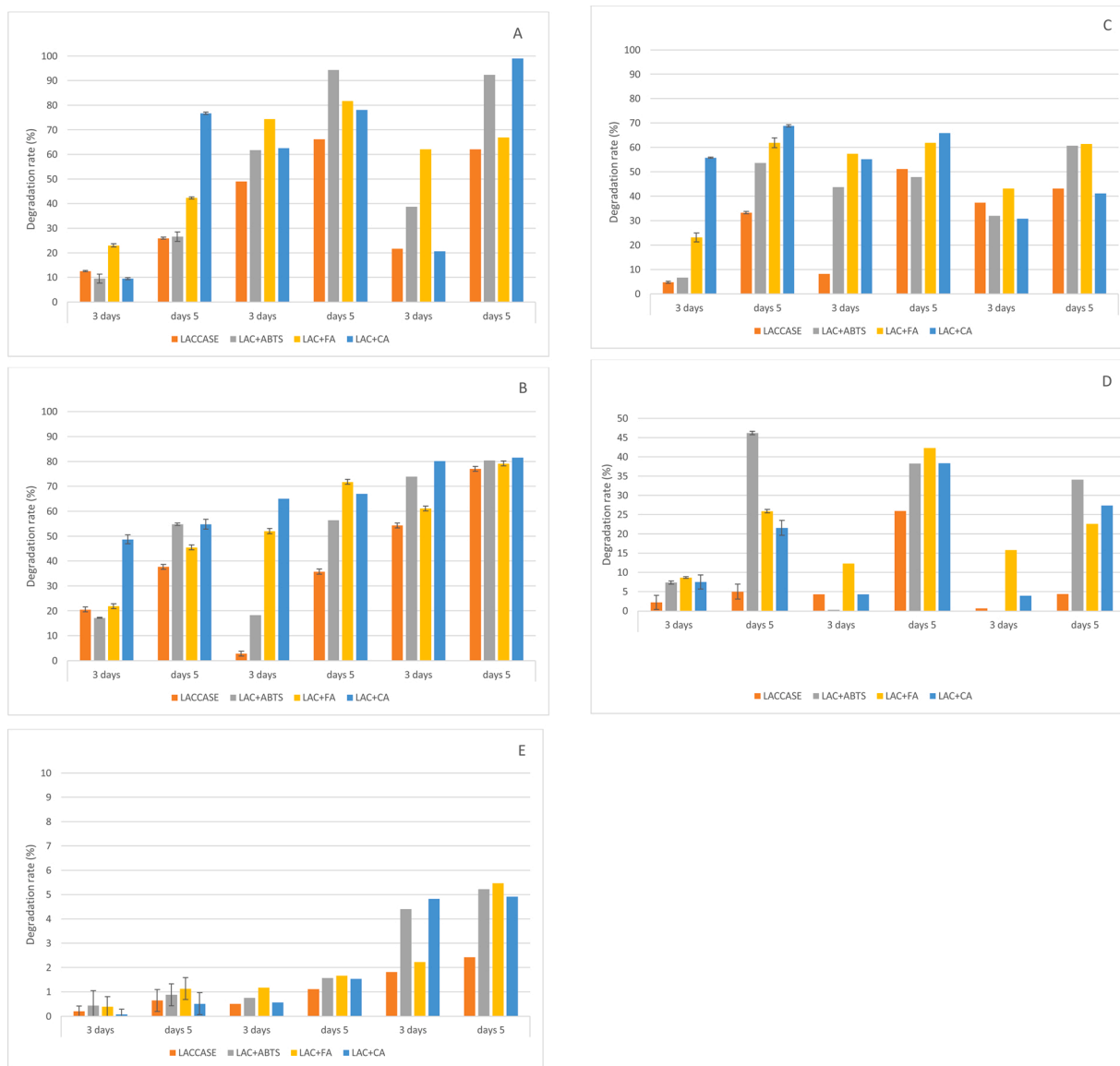
Fig. 4. PAH degradation from the soil by laccase in batch mode. (A) Pyrene, (B) Fluorene, (C) Chrysene, (D) Anthracene, (E) Benzo[a]pyrene. Degradation was performed at 30 °C, in the dark, using different concentration of PAH in Erlenmeyer flasks. The graphs are presented in a different scale.
