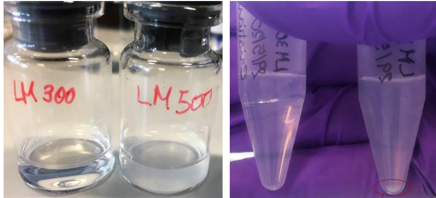
Figure 18 – Comparison between the L-Pmax to OL-HA ratio, evidencing the aggregation and sedimentation of the nanoparticles of the highest ratio (red circle). In each image, in the left is 0.3 ratio and in the 0.5 ratio.
