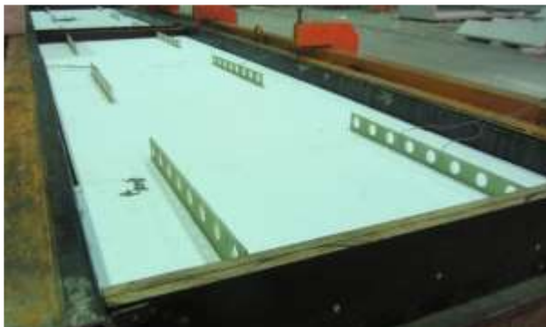
Figure 7 - Application of discontinuous GFRP connectors.
