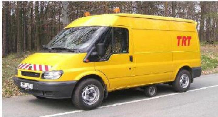
Figura 24 – Equipamento Tatra Runway Tester (TYROSAFE, 2008).
