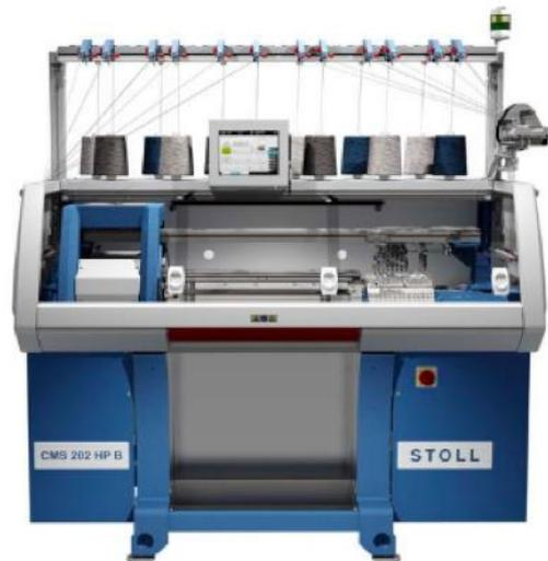
**Figura 2. 10.** Máquina de tricotar plana (<https://www.directindustry.com/pt/prod/stoll/product-180256-1776542.html>).
