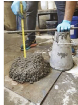
Fig. 4. Slump test of BFA5 mixture.
