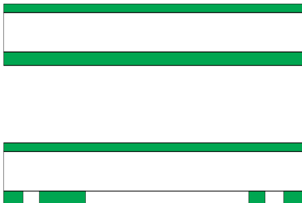
Figure A.1 Substrate (silicon wafer in white) with SiO 2 layers (green) deposited on the front and back sides (TOP). (B) Patterning of back side SiO 2 layer with mask #1. Layers thicknesses are not at scale.
