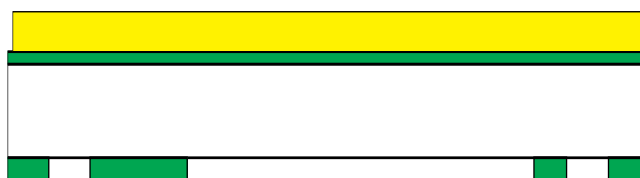
Figure A.2 Front side 9-10 μm thick polyimide layer (yellow) after curing and before patterning.
