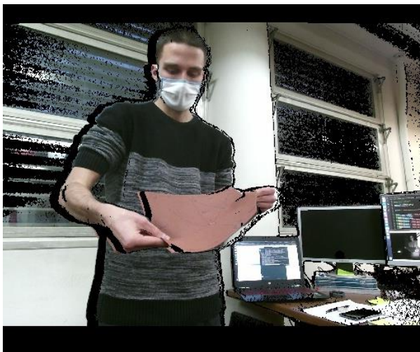
Figure 69- Inspection movement similar to "Torsion 1H" and the corresponding 3D pose estimation from ITP. A reference frame representing the hand's orientation is also attached to the hand.
