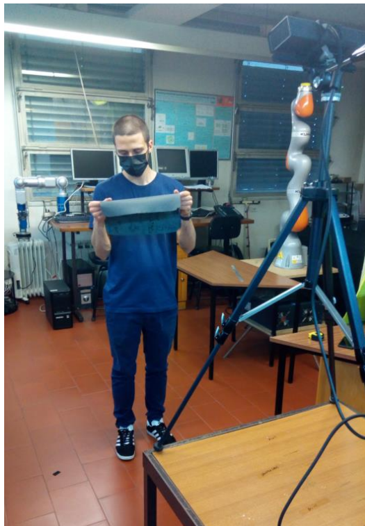
Figure 32 – Example of the inspection movements being “demonstrated” to the camera.
