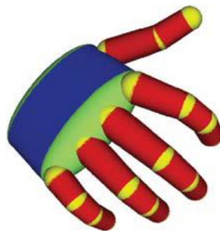
Figure 17- Hand model made of colour-encoded geometric primitives (yellow: elliptic cylinders, red: ellipsoids, green: spheres, blue: cones)[49].
