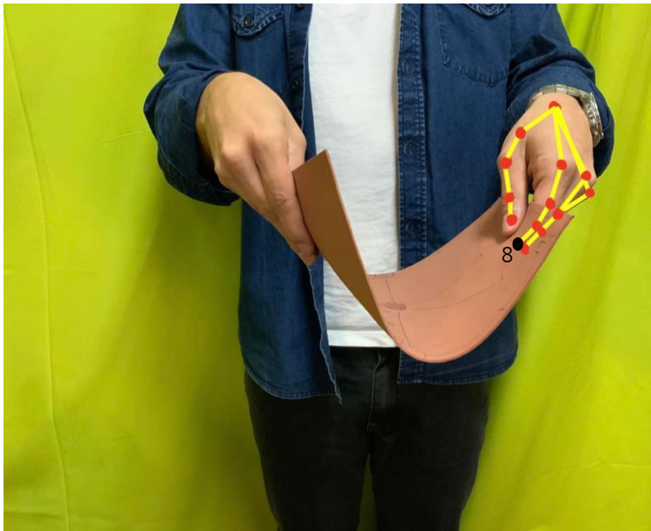
Figure 39 - Even with the detection of the hand skeleton in 2D, obtaining the depth value for point 8 would be impossible considering the occlusions. The depth value for that point would be measured to the surface of the leather piece.
