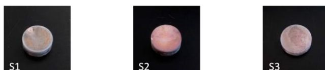
Figure 76 Photographs of S1, S2 and S3 samples of the third test group, obtained by Y-PSZ surface Au NP's irrigation and laser sintering procedure, and information on the adjusted laser parameters.
