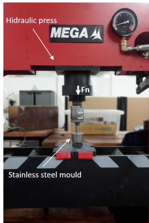
Figure 20 Hydraulic press equipment MEGA, Spain (micro fabrication and systems integration laboratory (CMEMS) of the Mechanical Engineering Department of University of Minho).~
