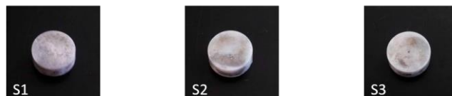
Figure 74 Photographs of S1, S2 and S3 samples of the second test group, obtained by Y-PSZ surface Au NP's irrigation and laser sintering procedure and information on the adjusted laser parameters
