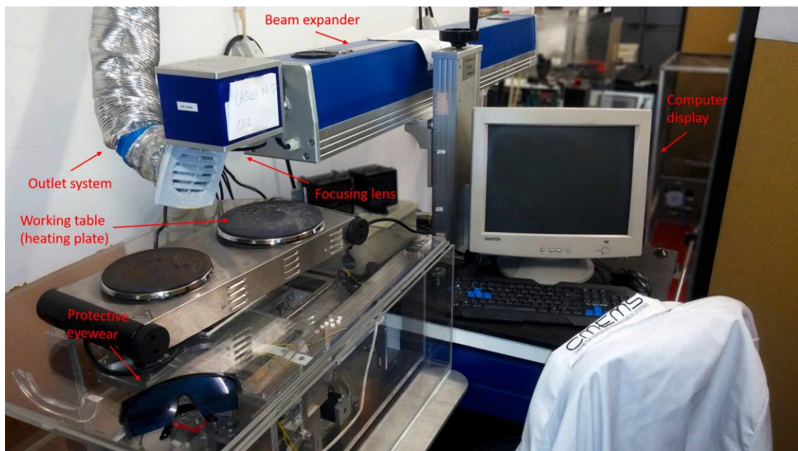
Figure 31 Laser system setup used in the experimental work (CMEMS Laboratory of the Mechanical Engineering Department of University of Minho).
