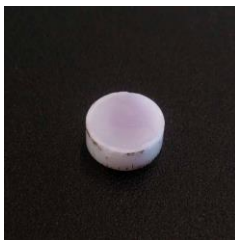
Figure 80 Photographs of the Y-PSZ sample after Au NP's spray and sintering in the oven procedure
