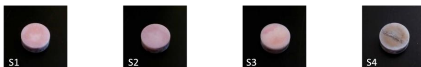
Figure 71 Photographs of S1, S2, S3 and S4 samples of the second testing group, obtained by Y-PSZ surface Au NP's irrigation and laser sintering procedure and information on the adjusted laser parameters
