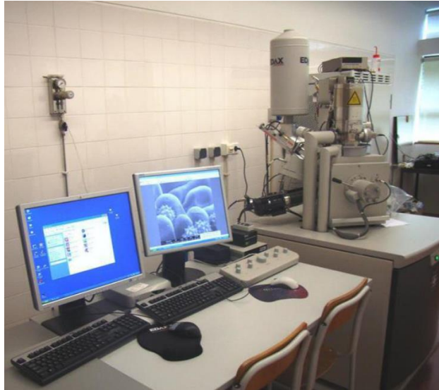
Figure 39 FEG-SEM; NOVA 200 Nano SEM, FEI, EUA, with integrated EDAX - Pegasus X4M (EDS/EBSD) (Laboratory for Materials Characterization Services of the University of Minho (SEMAT))
