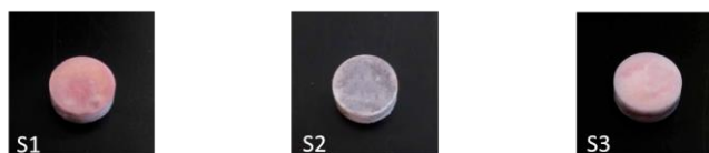
Figure 78 Photographs of S1, S2 and S3 samples of the fourth test group, obtained by Y-PSZ surface Au NP's irrigation and laser sintering procedure, and information on the adjusted laser parameters
