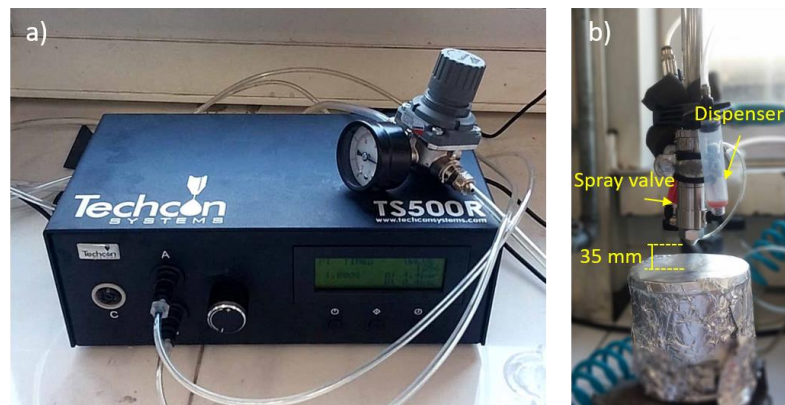
Figure 34 Spray equipment combined of: a) a Techcon Systems multi-purpose dispensing valve controller-TS500R, United Kingdom; b) respective precision spray valve-TS5540, same manufacturer (CMEMS Laboratory of the Mechanical Engineering Department of University of Minho).
