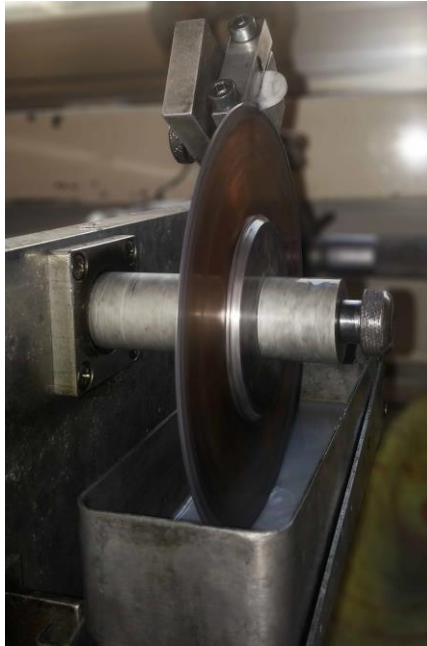
Figure 25 Diamond cutting disc used on the cross sectional cut of Y-PSZ samples (CMEMS Laboratory of the Mechanical Engineering Department of University of Minho).
