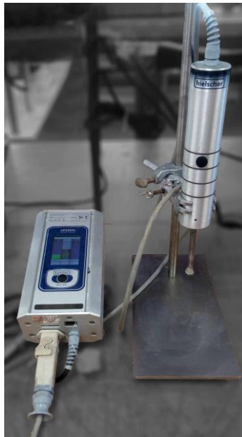
Figure 37 Ultrasonic processor, UP200St, Hielscher, Germany (CMEMS Laboratory of the Mechanical Engineering Department of University of Minho).
