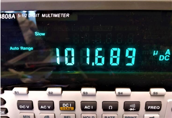
Figure 14 – Experimental excitation current using the implemented current source circuit.
