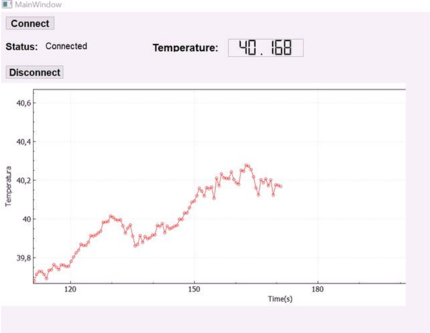
Figure 46 – Graphical interface showing the temperature value when a heating cycle between 39.7 and 40.3°C was applied.
