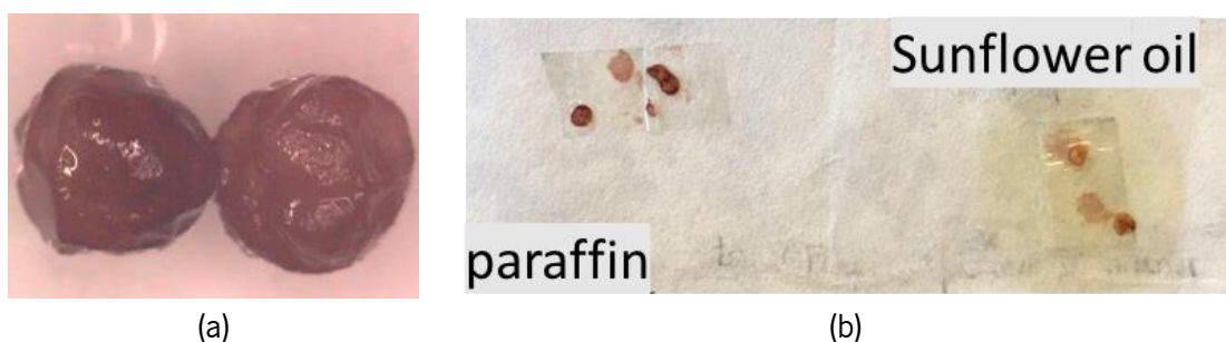
Figure i.9. (a) Amplified image of cellulose acetate capsules with UF as core (5%). (b) Photos of crushed cellulose acetate capsules with UF, synthesized with paraffin or sunflower oil as surfactants. The UF stained the filter and the capsules with sunflower oil also release the surfactant.
