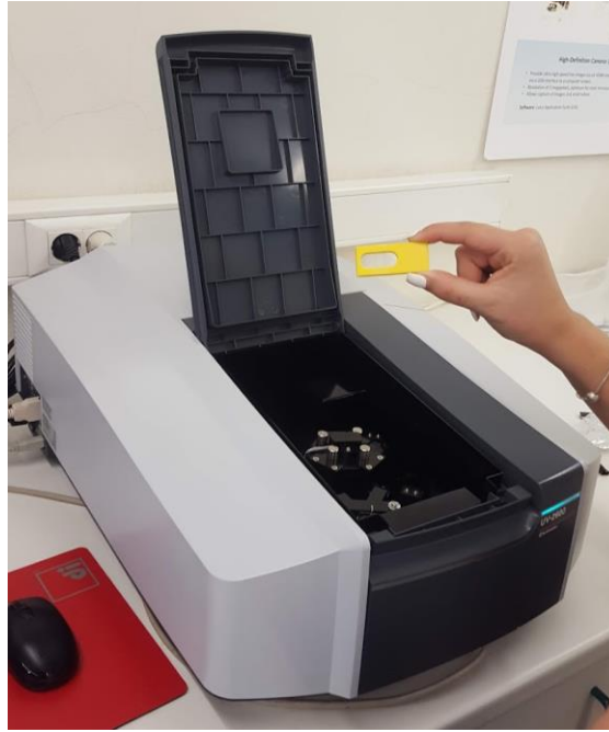
Figure 7. Spectrophotometer used for the transmittance tests. The yellow piece is an adapter used to place the PDMS sample in the equipment.
