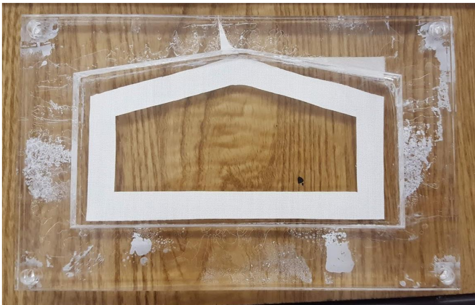
Figure 14. Acrylic mould to produce the PDMS films for the mask.
