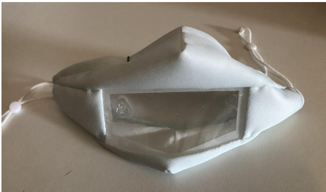
Figure 16. Mask prototype with fabric and PDMS made with a 5:1 mixing ratio and a 10% of recycled PDMS.
