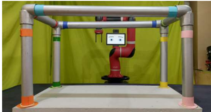
Figure 6.2: Structure consisting of one Base and eight colored parts: Green, Orange, Pink, Yellow (bottom) and Blue, Light Blue, Light Green, Red (top).
