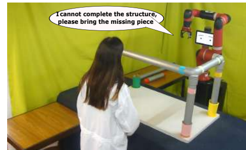
(b) Robot verbalizes to its co-worker that it is not possible to complete the structure without the missing item
