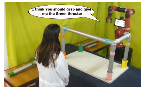
(b) Sawyer verbalizes to its co-worker that he should pass the Green piece to the robot
