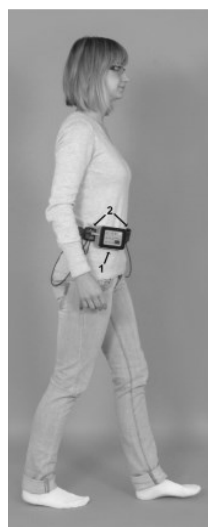
Figure 15. Vertiguard1-RT vibrotactile neurofeedback system with a main unit (1) and vibration pads (2). Taken from [41].
