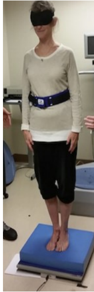
Figure 7. Participant wearing vibrotactile belt at the waist level and standing on the force platform. Taken from [37].
