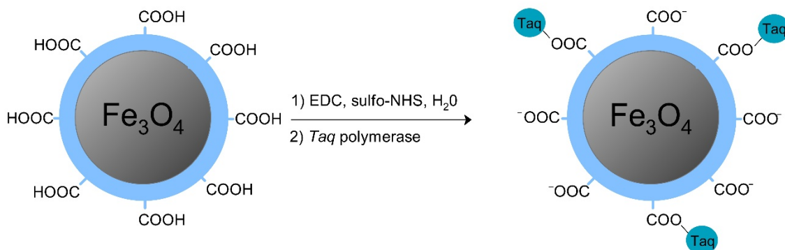
Figure 14. Schematic illustration of the coupling reaction of the carboxylic groups of the polyacrylic acid coating the magnetite nanoparticles to Taq polymerase.
