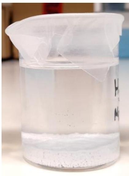
Figure 20 – NPs sedimentation in 2 mg/mL sonicated suspension after 24 h of stabilization.
