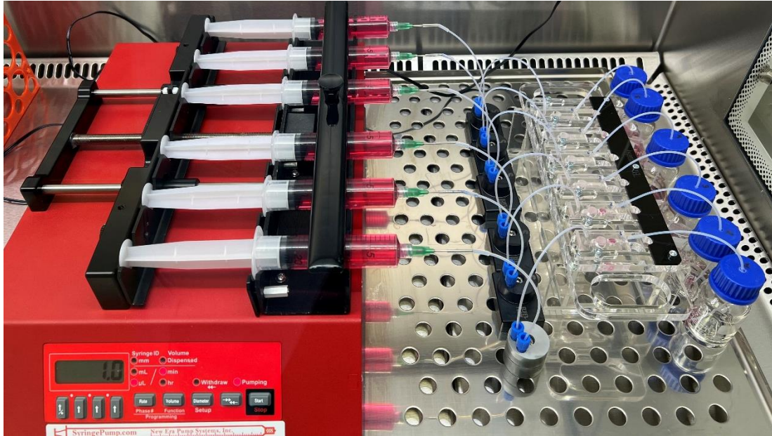
Figure 41 – Syringe pump-driven EoC set-up including bubble traps and the new support developed.
