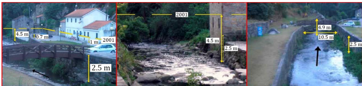
Figure 12. General view of several sectors in the Leça watershed and measurements of the 2001 flood. Adapted from [56].
