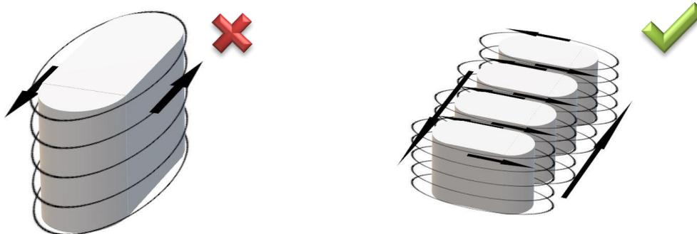
In case of the use four cells, we can observe the magnetic fields between the capacitor are in opposition, this reduces the resultant magnetic field.
