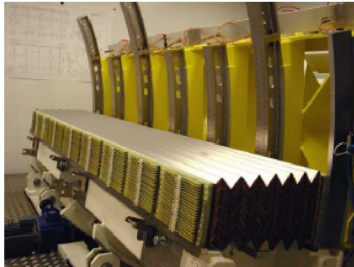
Figure 10: Photograph of a partially stacked barrel electromagnetic LAr module, where is visible the accordion geometry.
